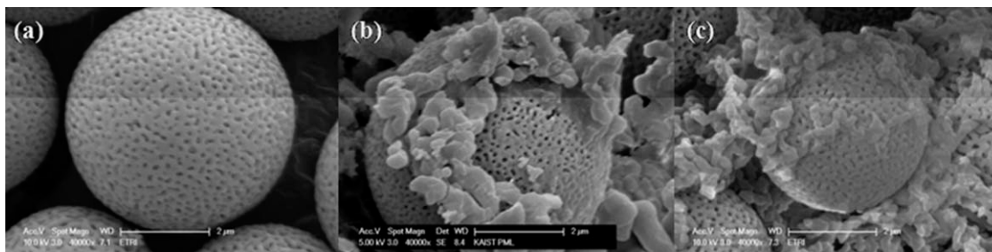
Figure 5. SEM images of the aminated SiO 2 (a), CSP with poly(styrene- b -cellulose 2,3- bis (3,5-dimethylphenylcarbamate)) prepared by “grafting from” method (b) and “grafting to” method (c).
